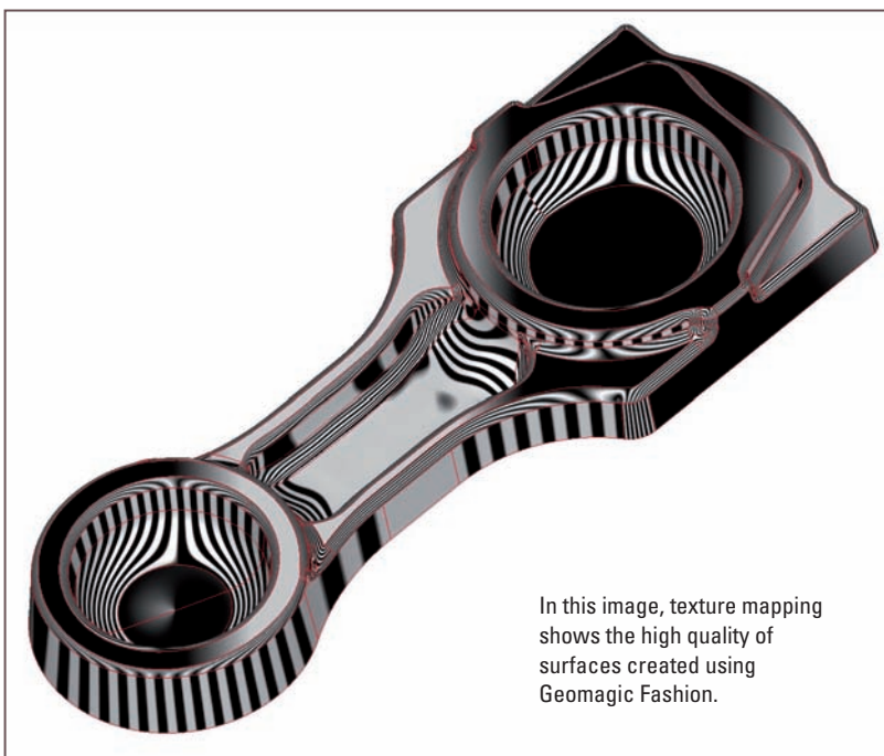
The new Geomagic Fashion module in Geomagic Studio 10 automatically extracts design intent from scanned physical objects. In this image, Geomagic Fashion classifies surfaces according to basic shapes such as planes, cylinder and freeform.
